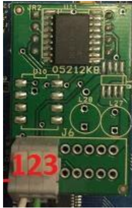
COM1 RS-232 Terminal Block (J6)
