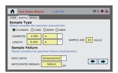
**Note:** Test rate of load control starts at 1% of machine capacity for all ASTM test options listed on the test standard menu screen.
