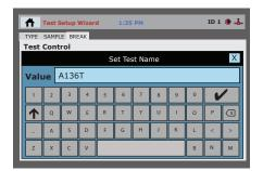
The machine begins to test using the preset loading rates. At sample failure the test stops, automatically retracting the load platen. When testing cylinders, a break-type pattern screen will open – select the break type. Then the Test Results Data screen appears storing the test data and load vs. time graph to memory. You are now ready to start the next test.
